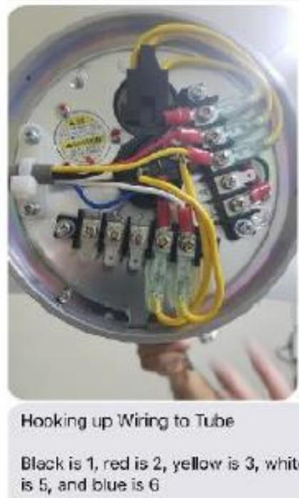
Figure 9: internal wiring of the tube.
