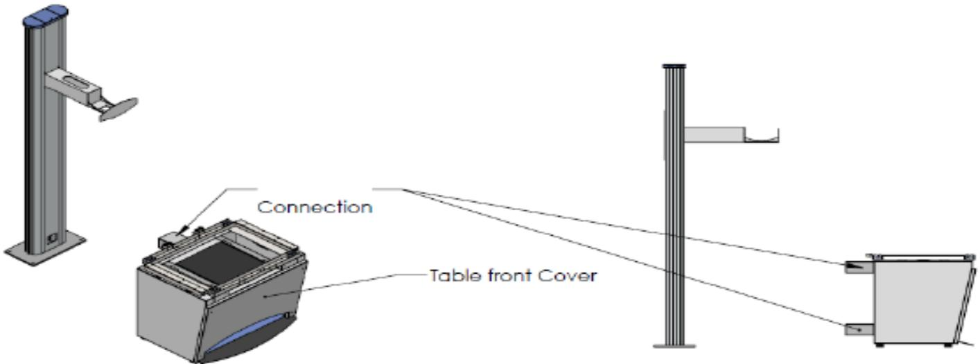
Figure 2: Table and the connection to the column.
